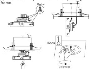
5. Disassembly process: one hand to hold the speaker assembly and push it up slightly, then use a hook to hook the edge of grill and rotate counterclockwise till the speaker assembly apart from the frame.
